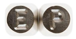
Reverse impression punches have a positive readable face to produce a negative indent - for use in forging or moulding applications, to produce a positive or readable inscription on a moulded or cast component
