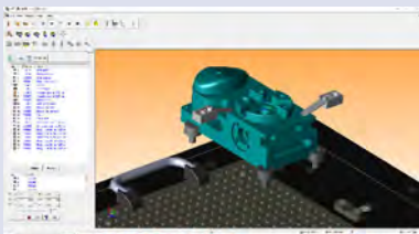
Applied support points and clamps
