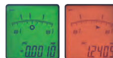
The display switches from green to red backlight if the upper or lower tolerance limit is exceeded
