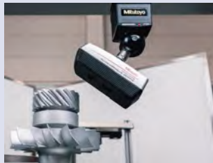
The flying spot type is capable of scanning difficult parts, such as this impeller, precisely and achieves highest scanning accuracy in the class.
