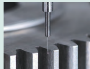
MPP-NANO Module 0.8 master gear measurement
