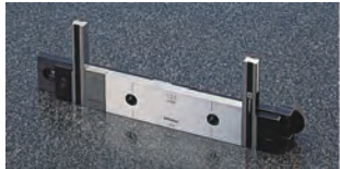
Holder B and C: Used for coupling two long gauge blocks together with other gauge blocks up to 35 mm (Holder B) or 140 mm Holder C). Also used for attaching jaws with two adapters. Holder B : 619032 (R max.= 90 mm- L= 126 mm) Holder C : 619033 (R max.= 200 mm- L= 236 mm)
