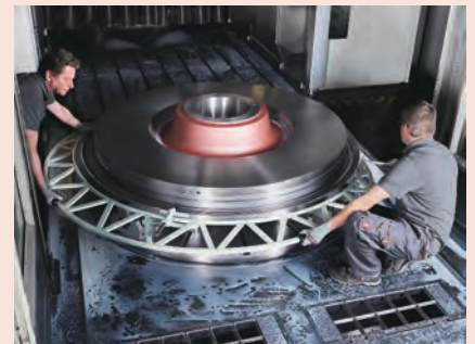
Application with adjustable stop on workpiece
