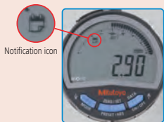
Calibration schedule warning
