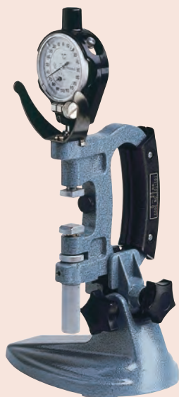
201-101 with optional accessories: stand 156-101-10 and dial indicator
