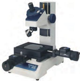
TM-505B fitted with optional digimatic micrometer heads
