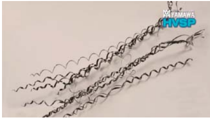
Ejected chips by large size taps
